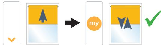
**Step 3:** Bring the shade to your desired upper limit. **PRESS & HOLD** both the **MY/STOP and DOWN** buttons until the shade begins to move down, then release. Stop the shade at the desired lower limit, adjust by pressing the **UP or DOWN** buttons.
