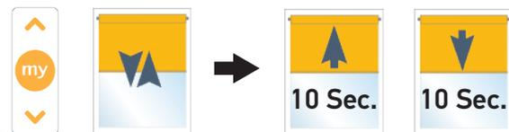
2) To increase the speed, **PRESS & HOLD** the **UP** button until the shade jogs. Repeat as needed.
