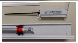
**6.** Insert the replacement motor into the headrail. Be sure to insert the feet of the motor into the slots at the bottom of the headrail.
