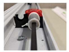
**8.** With the replacement motor fully inserted, tighten the screw to secure the foot of the motor.
