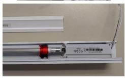
**4.** Loosen the screw securing the foot of the motor to the headrail.
