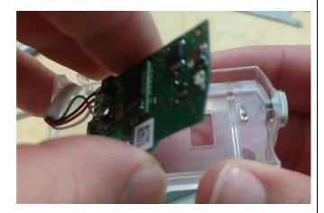
6. Remove the old push button by pushing out of the housing as shown below.
