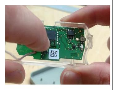
8. Insert the new push button into the housing by pressing into the housing as shown.
